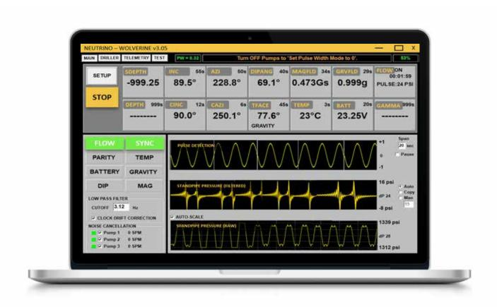
**Neutrino™** includes simple upgrade components for your downhole tool and surface system that allow you to receive data at 2 bits/sec. You get differentiation while your customers get to drill faster, save time, and stay on plan.
